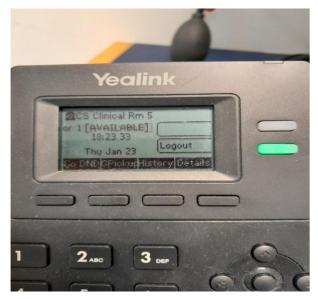
To log into the handset, press the green button and log out the current user (if necessary)
