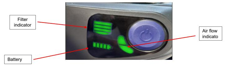
After a few seconds, the filter light & the battery light will go out and only the air flow indicator light will show.
