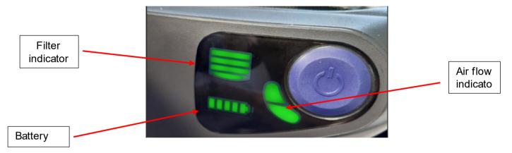
After a few seconds, the filter light & the battery light will go out and only the air flow indicator light will show.
